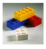
Shaping. ABS is distributed as pellets for moulding or extrusion. The material is normally available a rod or sheet in a range of colours.
